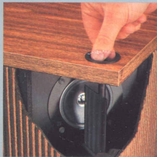
The Direct Energy Control changes the spatial properties of the 501 system by controlling the radiation pattern of the outward-firing tweeter above 3 kHz.
